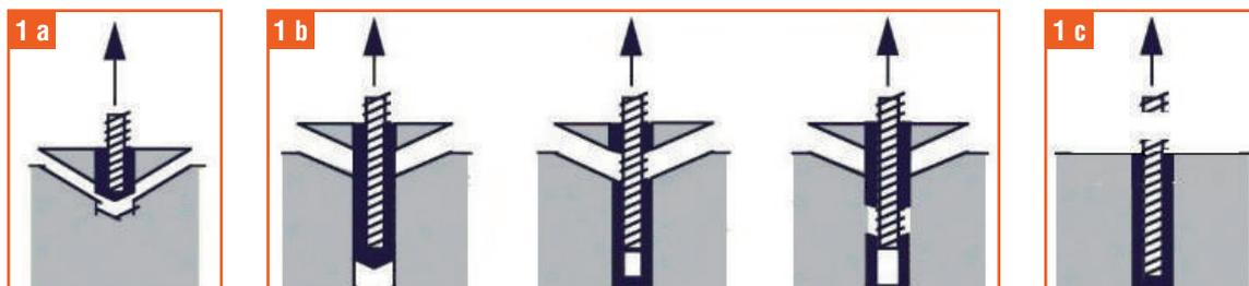
**Fig. 1** – Modalità di rottura (da Cook, Kunz, Fuchs e Konz, 1998, "Behavior and Design of Single Adhesive Anchors under Tensile Load in Uncracked Concrete", ACI Structural Journal, V.95, No. 1).
